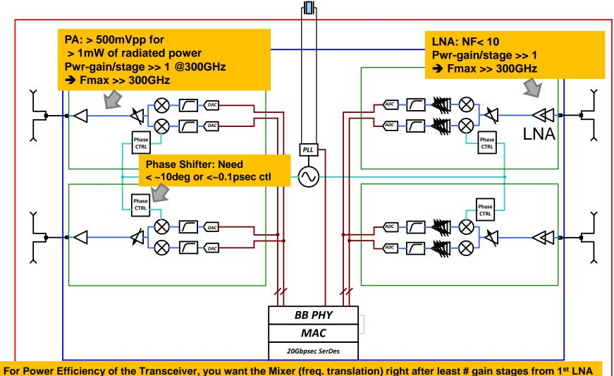
→ MOS passive Mixer Noise Figure is also very critical and also improves with higher Fmax, and lower Cgs
