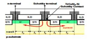
Shallow trench separated Schottky barrier diode.
